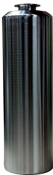
6. Nuclear waste container. The cylinder is made of stainless steel with a height of 1.35 m and diameter of 0.43 m. It contains about 400 kg of borosilicate glass which traps the waste. The total weight is about 500 kg.
