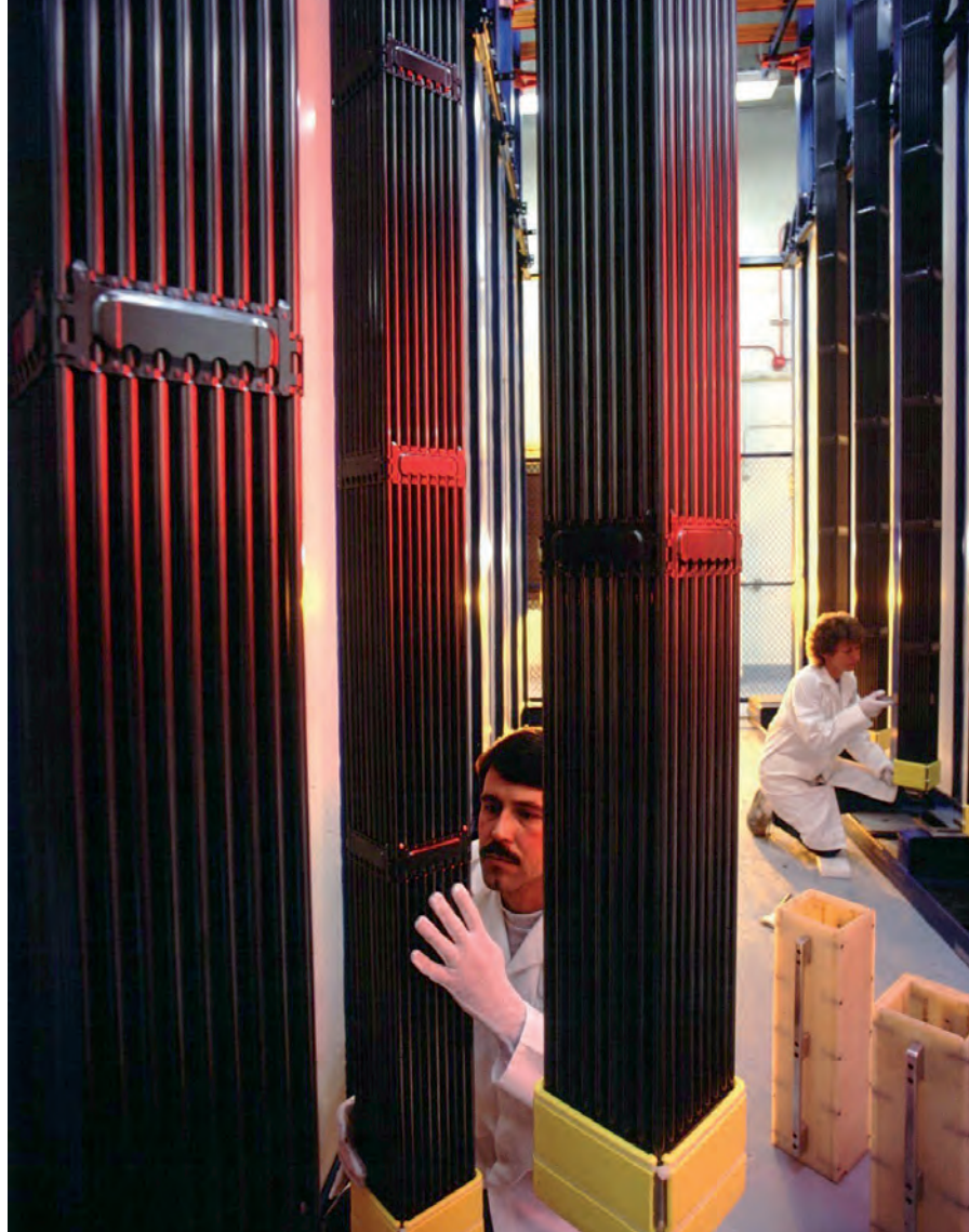
4. Nuclear fuel assembly of a pressurized water reactor with control rod. The grids provide mechanical support to maintain the 264 fuel rods.
