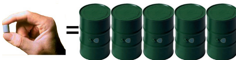
1. Image showing the size of an enriched uranium oxide pellet used in the production of nuclear fuel in a pressurized water reactor. For a given amount of energy, nuclear power uses 100,000 times less raw material than fossil fuels (oil, gas or coal).
