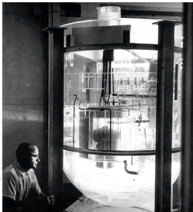
Scale model (1/6) of the Molten Salt Reactor Experiment (MSRE) at Oakridge (USA). The MSRE diverged on 1 June 1965, and reached full power (7500 kW) in May 1966.
