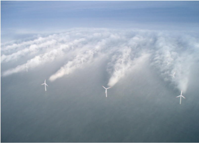
4. Offshore wind farm, where local weather conditions led to condensation revealing part of the turbines' wake.
